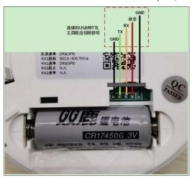
$2\sqrt{15200}$  Open the serial port software, and set the Baud to 115200,8, n, 1
