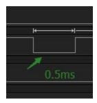
3. preamble :first high level 0.5ms then low level 0.5ms, loop 5 times
