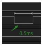
6. Data packet: The data packet follows the standard Manchester encoding. 10 represents 1,01 represents 0. H\_id (the highest bit is 0 means no data, the highest bit 1 means there is data after 1byte) + data length (1byte) + data (n byte) + checksum (data addition) (1byte)
